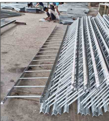
Cable Tray & Ladders
